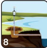
Insert the connector marked "Control" in the Control box (provided) and Connect the electricity using connector (provided) and fix the Pipe carefully using bricks, stones and soils. (Figure 9) Make sure the pipe is firmly fixed in the ground and the connector box is visible. Fix the control box using bolts (Provided) on the pipe.
